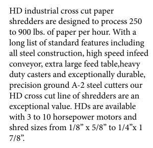
7.5 Motor Output In HP Infeed Width In Inches Shred Width in Inches 1/8" x 1 1/2" Throughput (Lbs per hour) 450-650 1725 Weight (lbs) Speed (FPM) Size L/W/H in Inches 59/36/47.5 Standard Features Precision Ground A-2 Steel Cutters, Bag Holder, Extra Large Feed Table, Heavy Duty Casters Available Options Auto Lubrication, Output Conveyor, Cart Tipper \* Single & Three Phase Power - Single Phase
